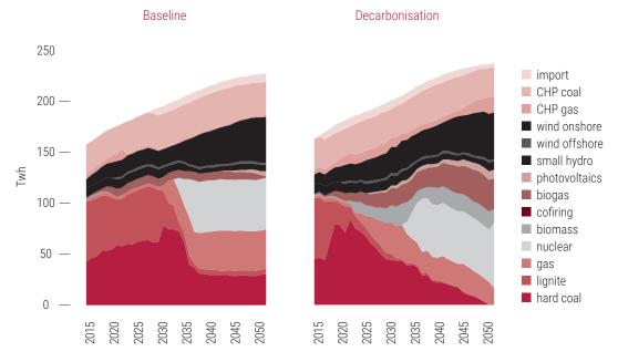
Figure 3.4. The optimal electricity mix under the baseline (left) and decarbonisation (right) pathways, assuming low costs of intermittent RES
