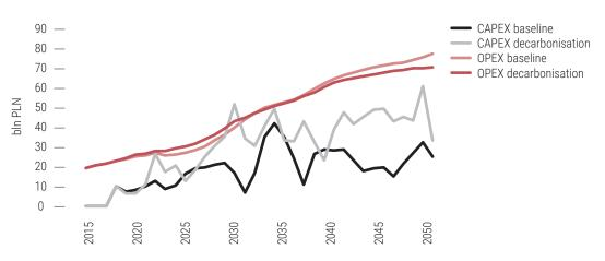
Figure 3.11. CAPEX and OPEX under the decarbonisation and baseline pathways, assuming that nuclear technology is not available
