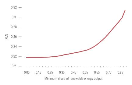
Figure 5.1. Levelised cost of electricity in PLN per kWh for different levels of minimum required share of renewable energy output
